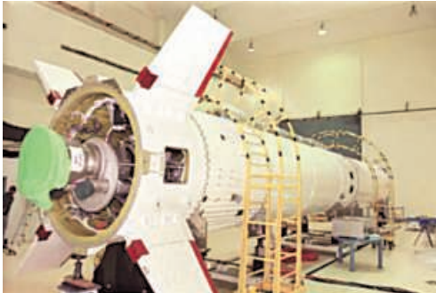
Test vehicle for characterisation of Crew Escape System ready at SDSC PHOTO: ISRO
